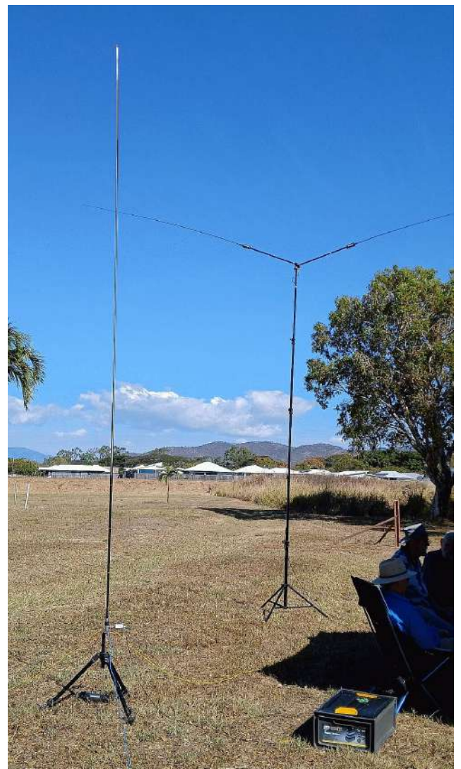
The Tubby 40m vertical and 40m loaded dipole antennas deployed near the Bomb Crater
